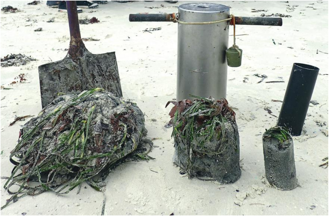
Plate 12. Demonstration of 'seagrass-with-sediment' methods, showing sod with shovel (left) and two sizes of plugs with corers (centre and right).
